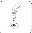
Remove the vial from the sample chamber.
