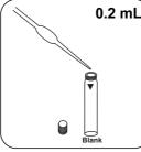
Prepare two reaction vials. Put 0.2 mL deionised Mark one as a blank.
