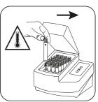
Remove the vial from the thermoreactor. (Note: vial will be hot!)
