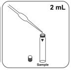
Prepare two reaction vials. Put 2 mL deionised water Put 2 mL sample in the Mark one as a blank.
