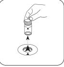
Remove the vial from the sample chamber.
